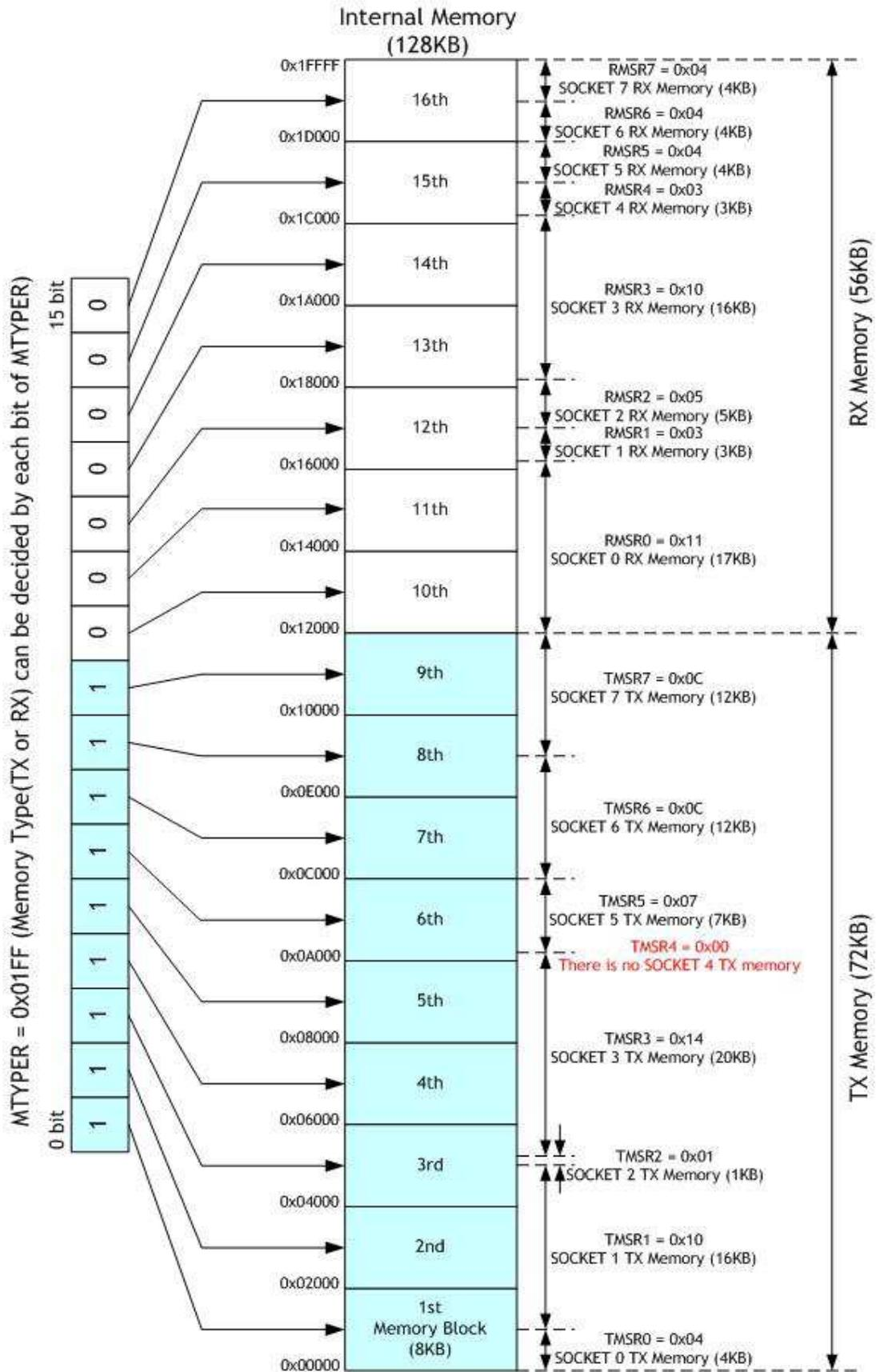
**Fig 8. Allocation Internal TX/RX memory of SOCKETn**
