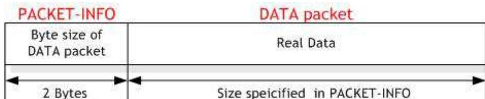
**Fig 11. The received TCP data format**
