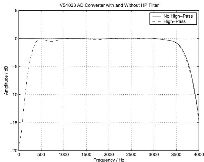
Figure 15: ADPCM Frequency Responses with 8 kHz sample rate.
