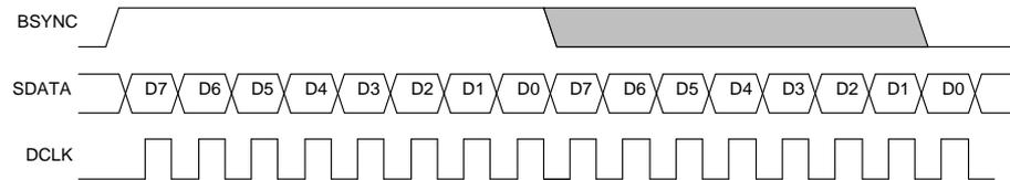
Figure 5: BSYNC Signal - two byte transfer.
