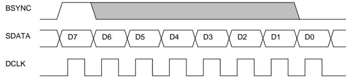
Figure 4: BSYNC Signal - one byte transfer.
