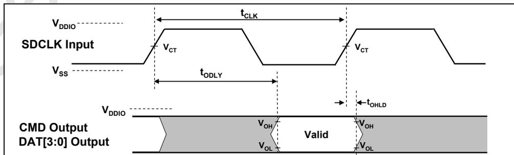
**Figure 6-16 : Output Timing of Fixed Data Window**
