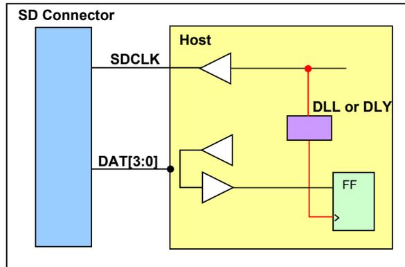
Figure C- 1 : Delayed Internal Clock Method
