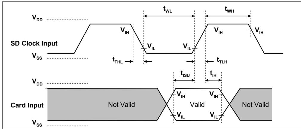
**Figure 6-8: Card Input Timing (Default Speed Card)**
