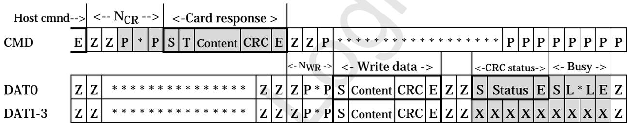
**Figure 4-31: Timing of Single Block Write Command**
