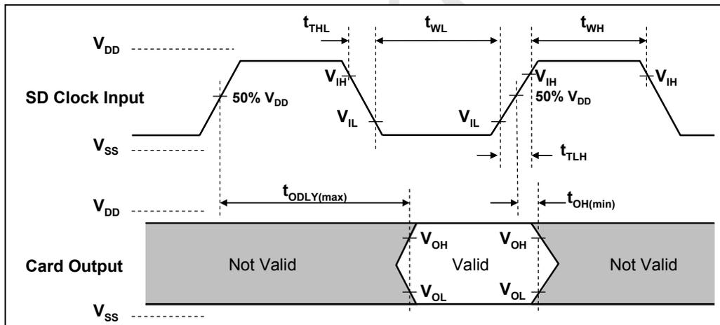
**Figure 6-11: Card Output Timing (High Speed Mode)**
