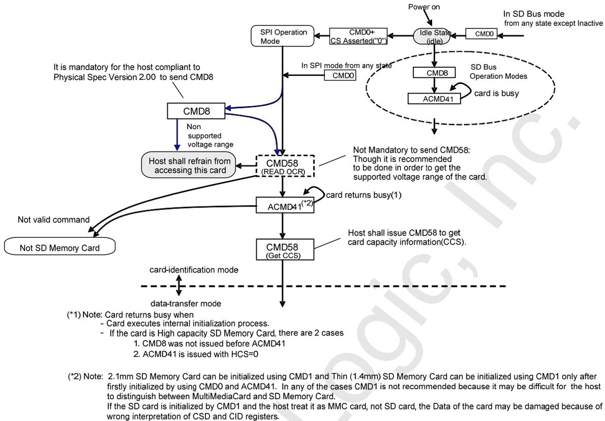
**Figure 7-1 : SD Memory Card State Diagram (SPI mode)**
