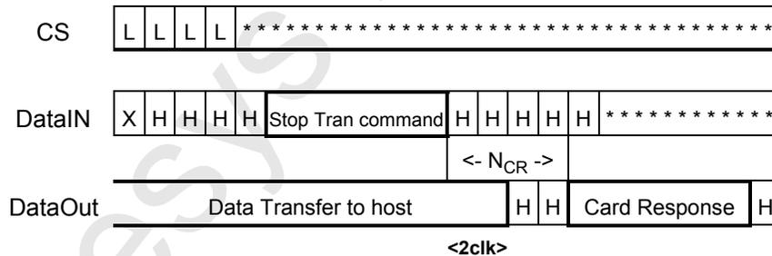
**Figure 7-18: Stop Transmission in Read Multiple Block**
