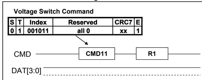
**Figure 4-9 : Voltage Switch Command**
