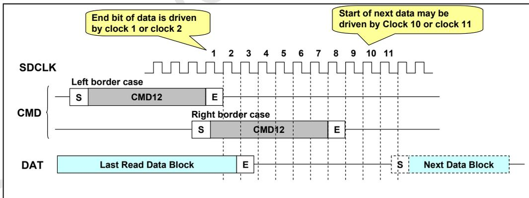
**Figure 4-40 : Border Timing of CMD12 in Read Operation**
