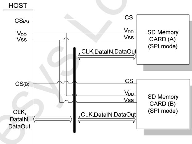
**Figure 3-2: SD Memory Card System (SPI Mode) Bus Topology**
