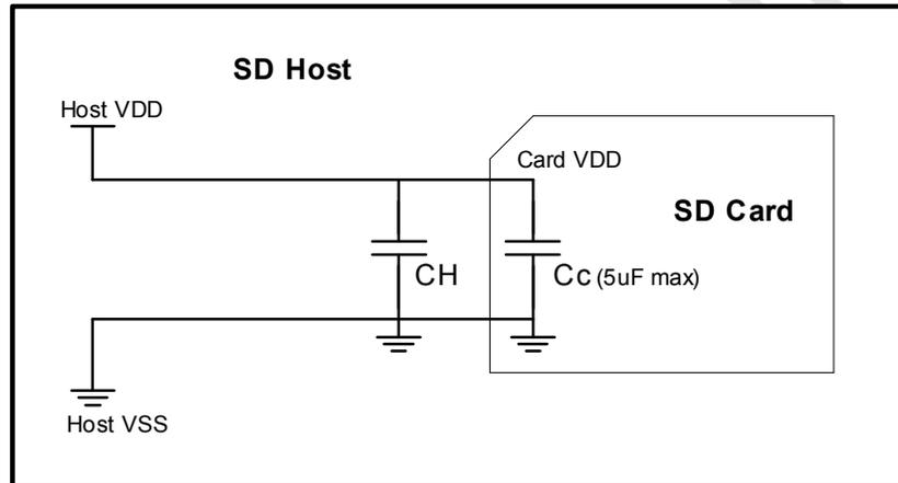
**Figure E- 1 : Capacitance Connected to Power Line**
