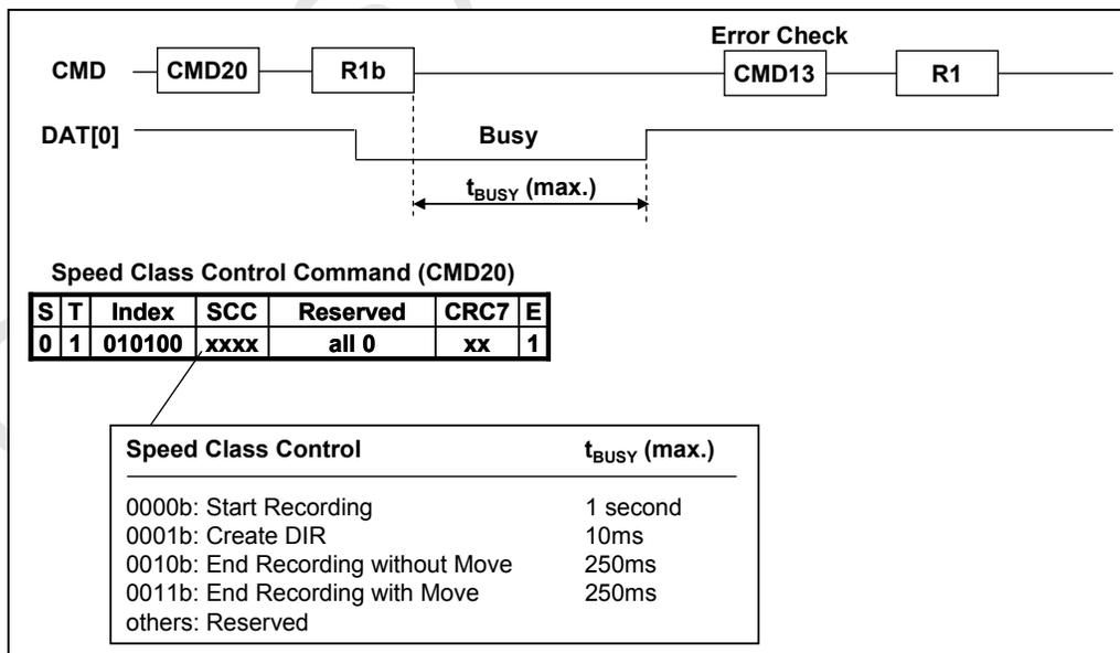
**Figure 4-53: Timing and Command Argument of CMD20**
