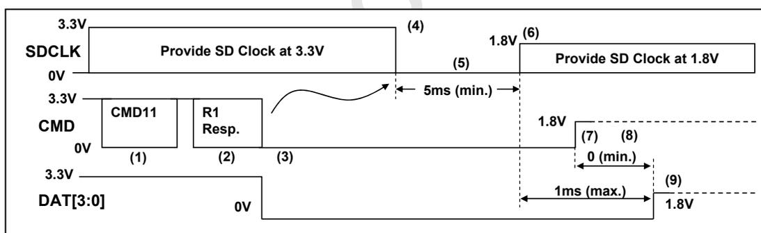
**Figure 4-7 : Signal Voltage Switch Sequence**
