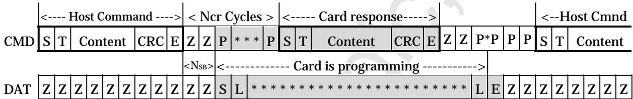
**Figure 4-36: Stop Transmission received after Last Data Block. Card becomes busy.**
