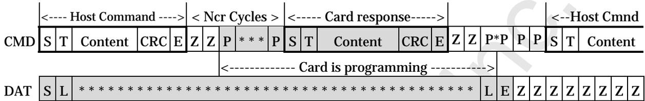
**Figure 4-35: Stop Transmission received after Last Data Block. Card is busy programming.**
