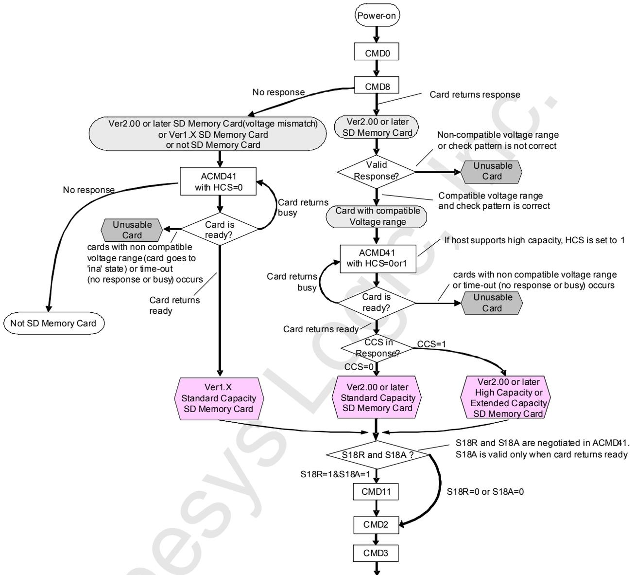
**Figure 4-2: Card Initialization and Identification Flow (SD mode)**
