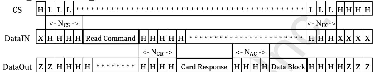
**Figure 7-17: Read Single Block Operations - Bus Timing**
