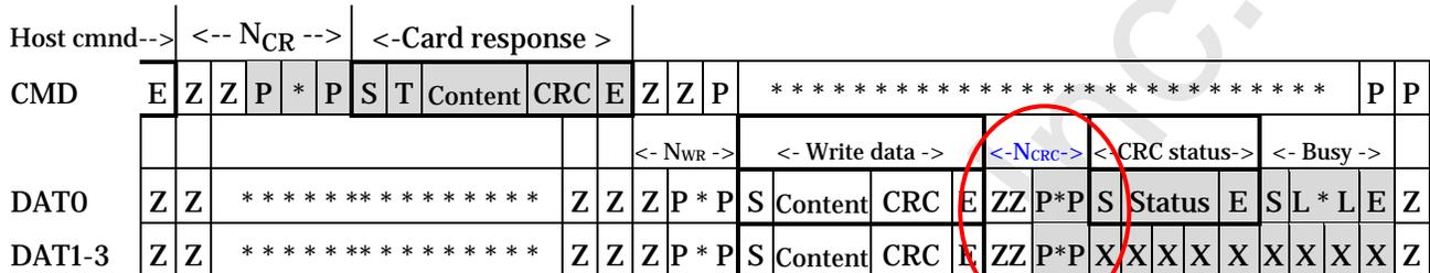
**Figure 4-37 : Timing of Single Block Write Command**
