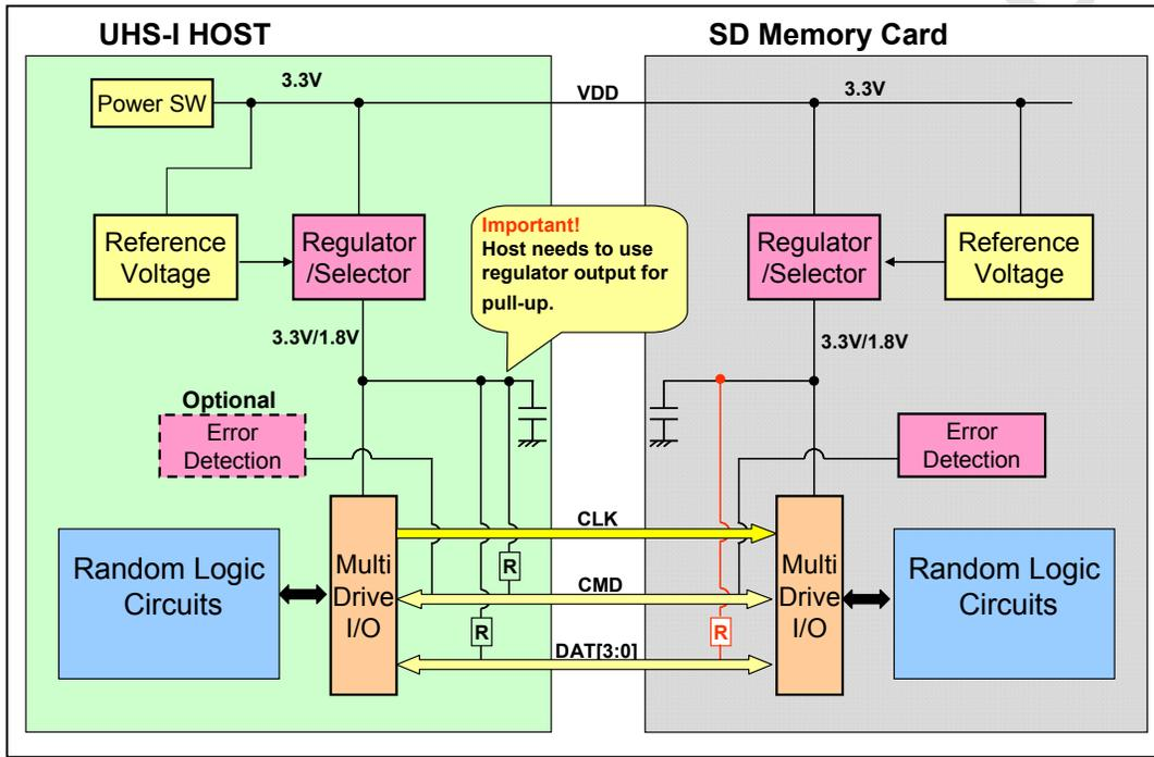
Figure 4-12 : An Example of UHS-I System Block Diagram
