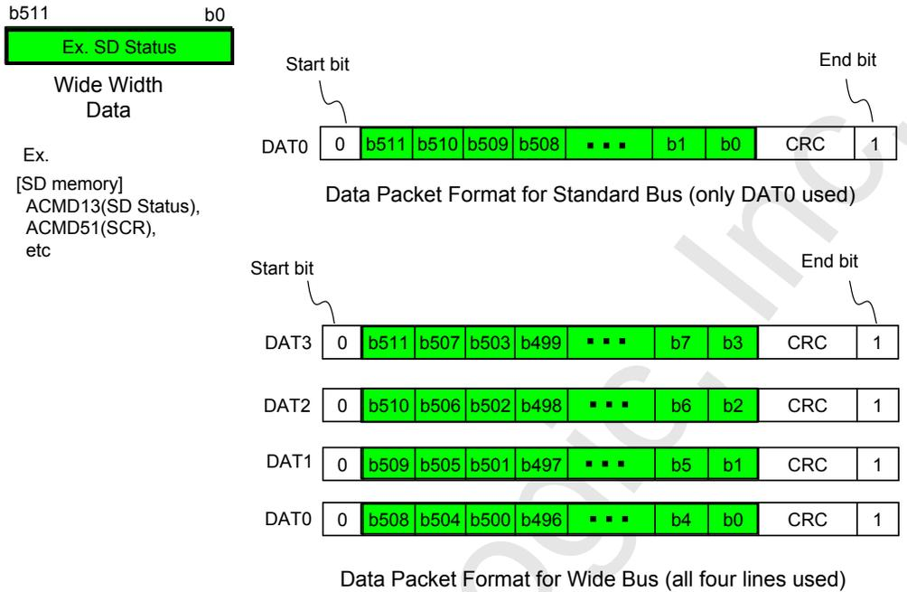
**Figure 3-9: Data Packet Format - Wide Width Data**
