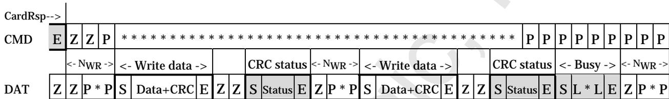
**Figure 4-32: Timing of Multiple Block Write Command**
