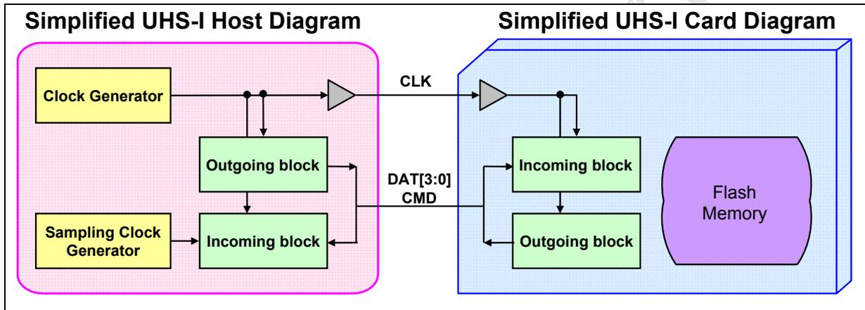
Figure 3-15 : Host and Card Block Diagram
