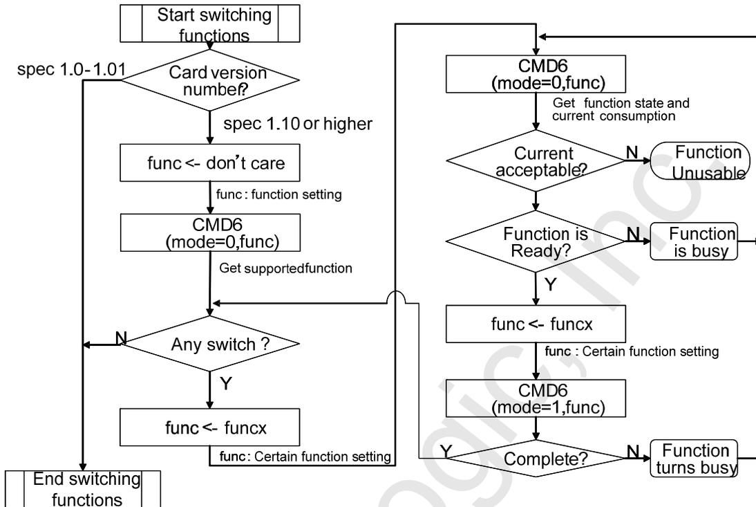
**Figure 4-19: Switching Function Flow**
