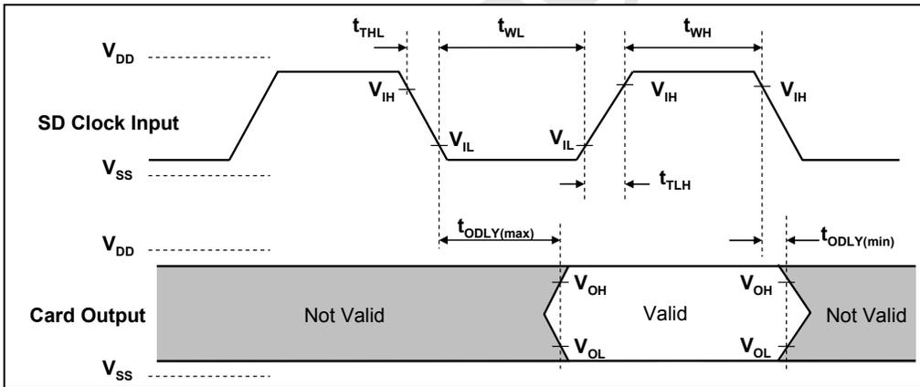
**Figure 6-9: Card Output Timing (Default Speed Mode)**
