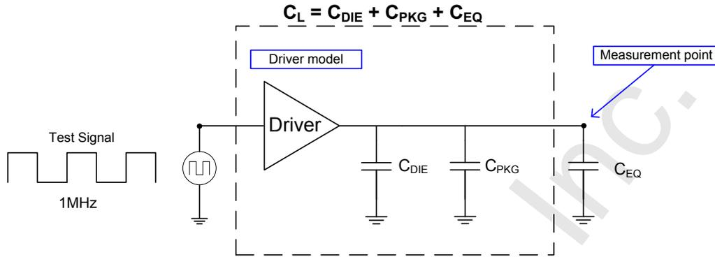
**Figure 6-12 : Outputs Test Circuit for Rise/Fall Time Measurement**
