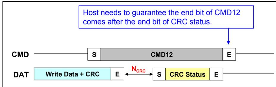
**Figure 4-39 : Border Timing of CMD12 in Write Operation**
