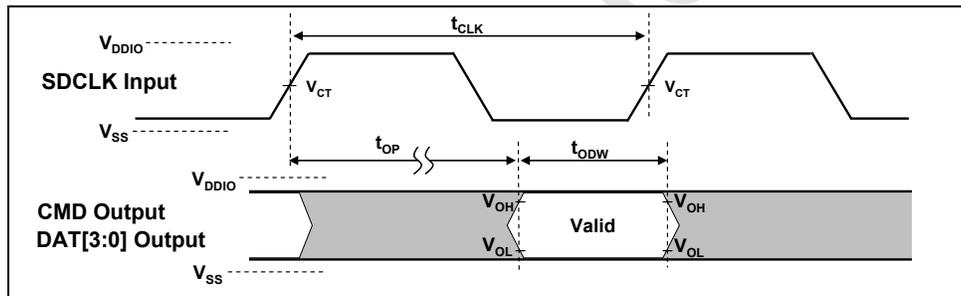
**Figure 6-17 : Output Timing of Variable Data Window**
