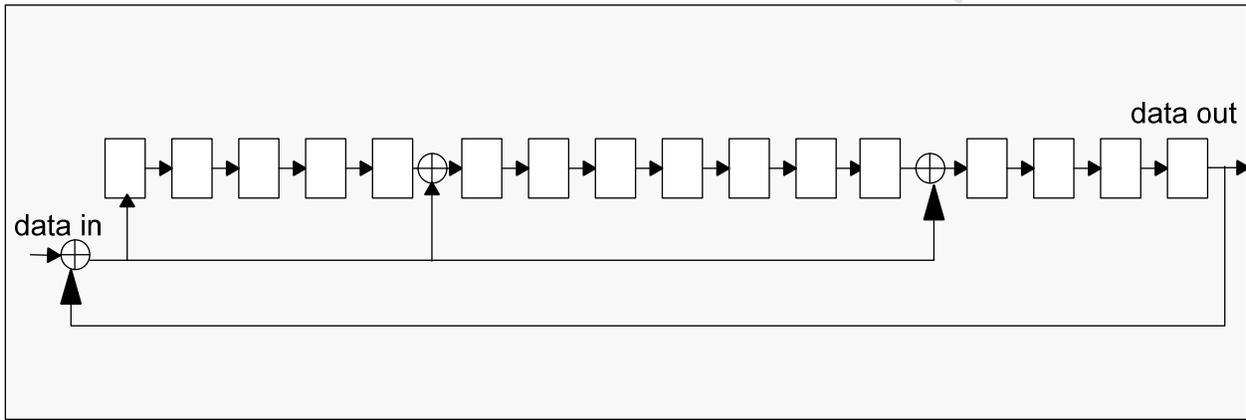
**Figure 4-21: CRC16 Generator/Checker**
