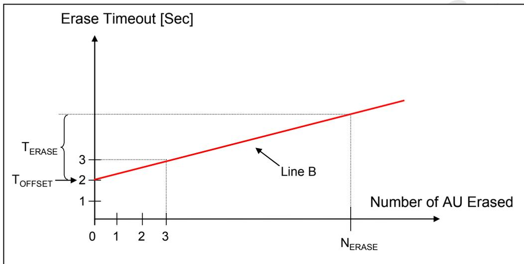
**Figure 4-56: Example Erase Characteristics (Case 2  $T_{OFFSET}=2$ )**
