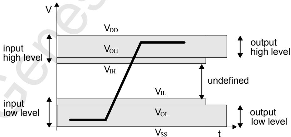
**Figure 6-7: Bus Signal Levels**
