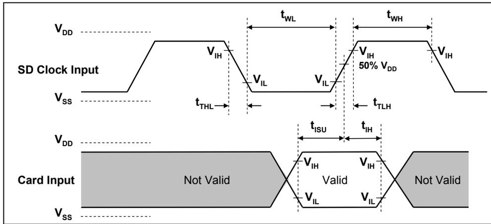
**Figure 6-10: Card Input Timing (High Speed Card)**
