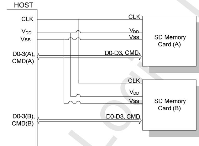
Figure 3-1: SD Memory Card System Bus Topology
