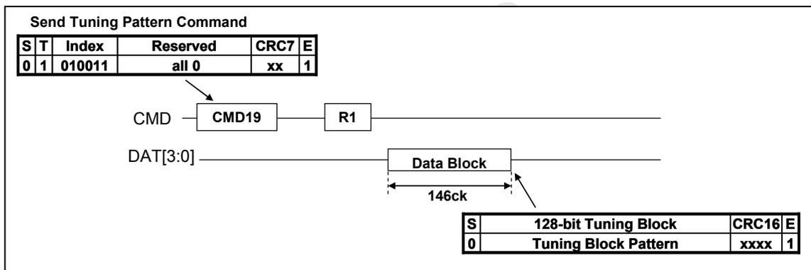
**Figure 4-10 : Send Tuning Pattern Command**
