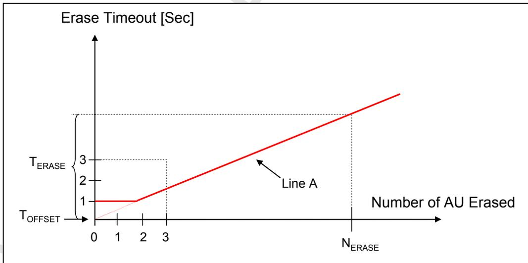
Figure 4-55: Example Erase Characteristics (Case 1  $T_{OFFSET}=0$ )
