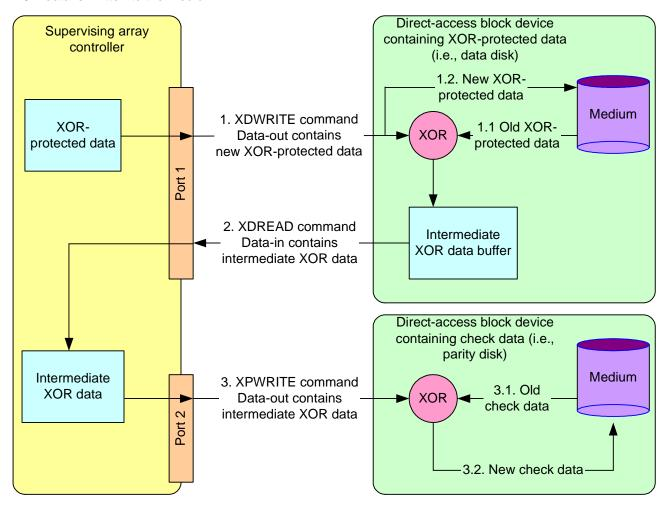
Figure B.1 — Update write operation (storage array controller supervised)
