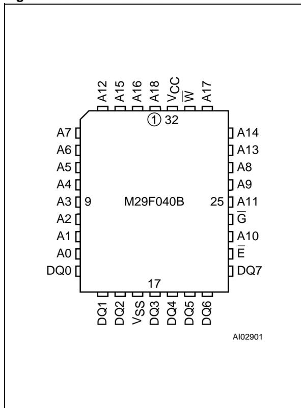
**Figure 3. TSOP Connections**
