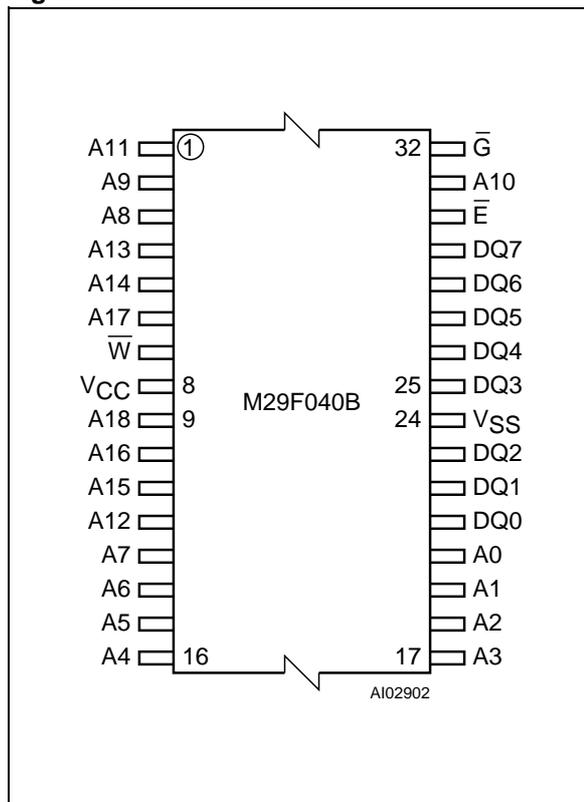
**Figure 4. PDIP Connections**
