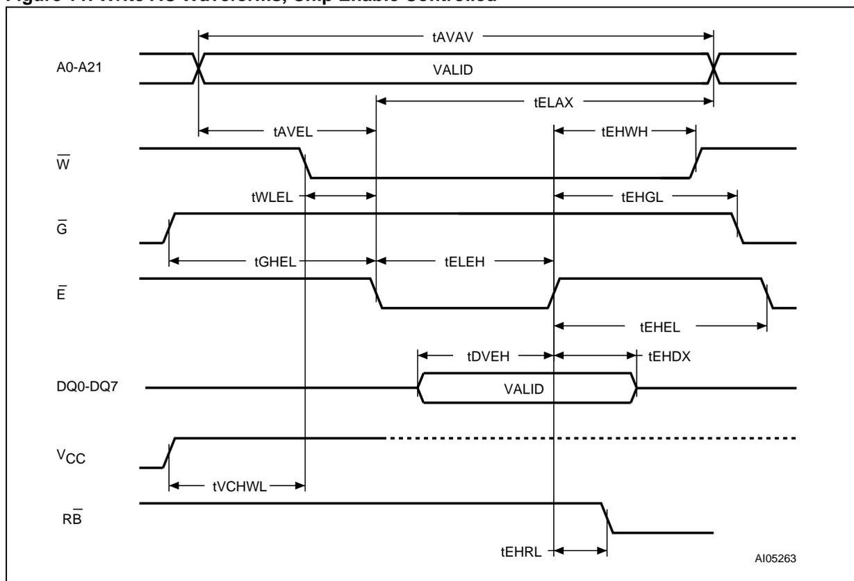
Table 12. Write AC Characteristics, Chip Enable Controlled
