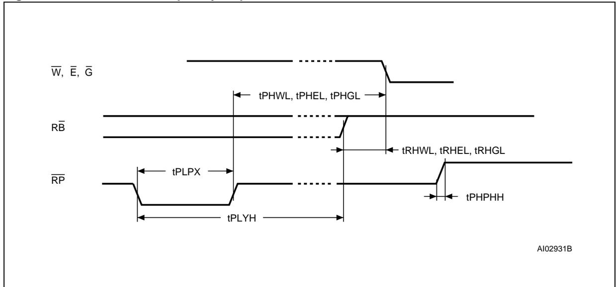
Table 13. Reset/Block Temporary Unprotect AC Characteristics
