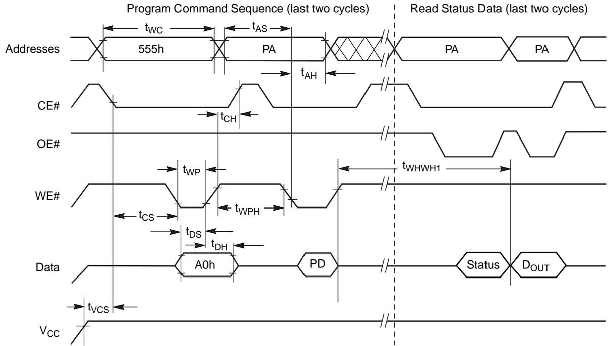
Note: PA = program address, PD = program data, D<sub>OUT</sub> is the true data at the program address.
