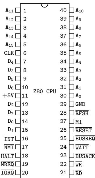
A<sub>15</sub> – A<sub>0</sub> Address bus (output, active high, 3-state). This bus is used for accessing the memory and for I/O ports. During the refresh cycle the IR register is put on this bus.
