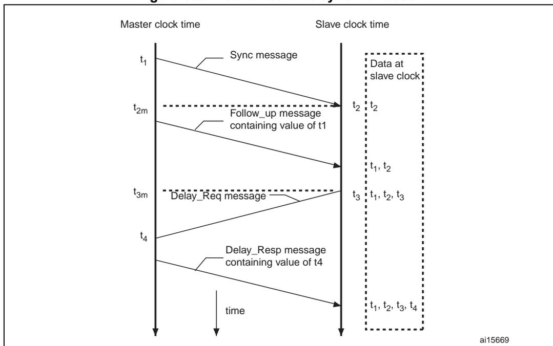
1. The master broadcasts PTP Sync messages to all its nodes. The Sync message contains the master’s reference time information. The time at which this message leaves the master’s system is  $t_1$ . For Ethernet ports, this time has to be captured at the MII.
