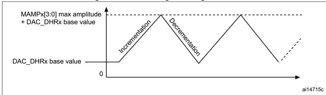
**Figure 55. DAC conversion (SW trigger enabled) with triangle wave generation**
