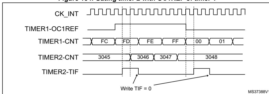
In the example in [Figure 154](#), the Timer 2 counter and prescaler are not initialized before being started. So they start counting from their current value. It is possible to start from a given value by resetting both timers before starting Timer 1. You can then write any value
