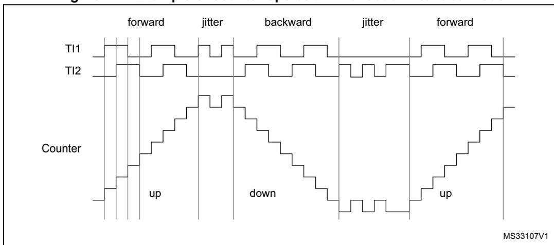
Figure 148 gives an example of counter behavior when TI1FP1 polarity is inverted (same configuration as above except CC1P=1).
