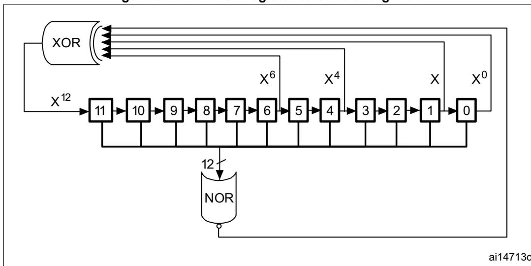
The LFSR value, that may be masked partially or totally by means of the MAMPx[3:0] bits in the DAC\_CR register, is added up to the DAC\_DHRx contents without overflow and this value is then stored into the DAC\_DORx register.
