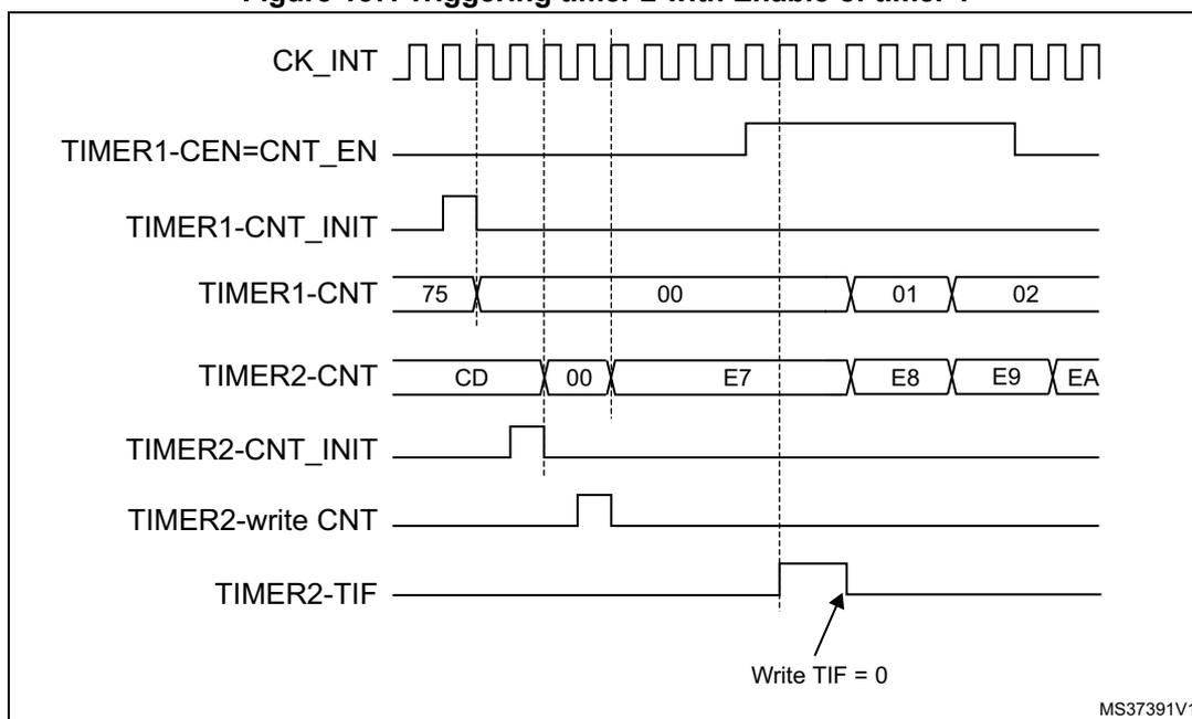
**Starting 2 timers synchronously in response to an external trigger**
