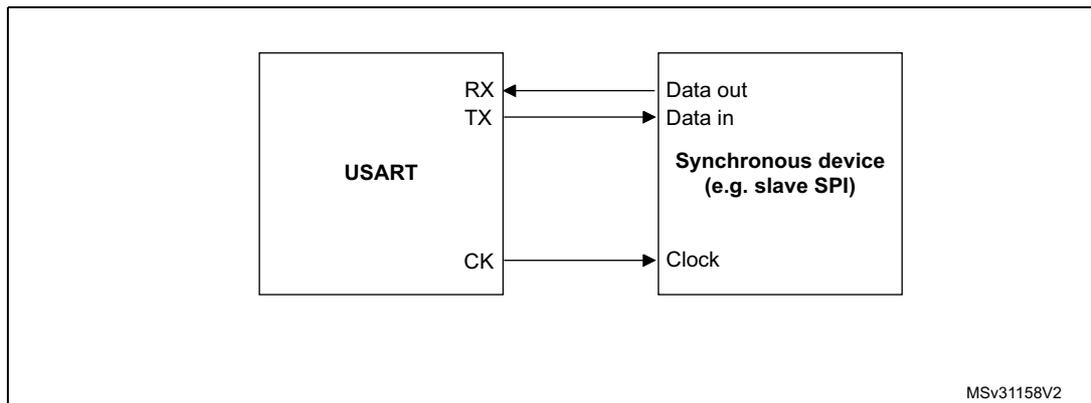
Figure 235. USART data clock timing diagram (M=0)
