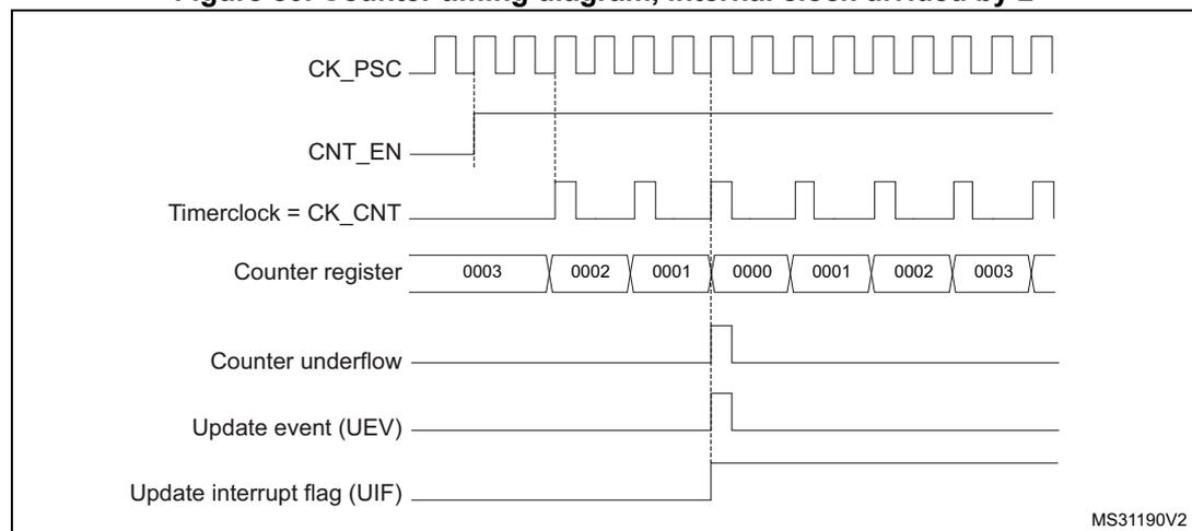
**Figure 81. Counter timing diagram, internal clock divided by 4, TIMx\_ARR=0x36**
