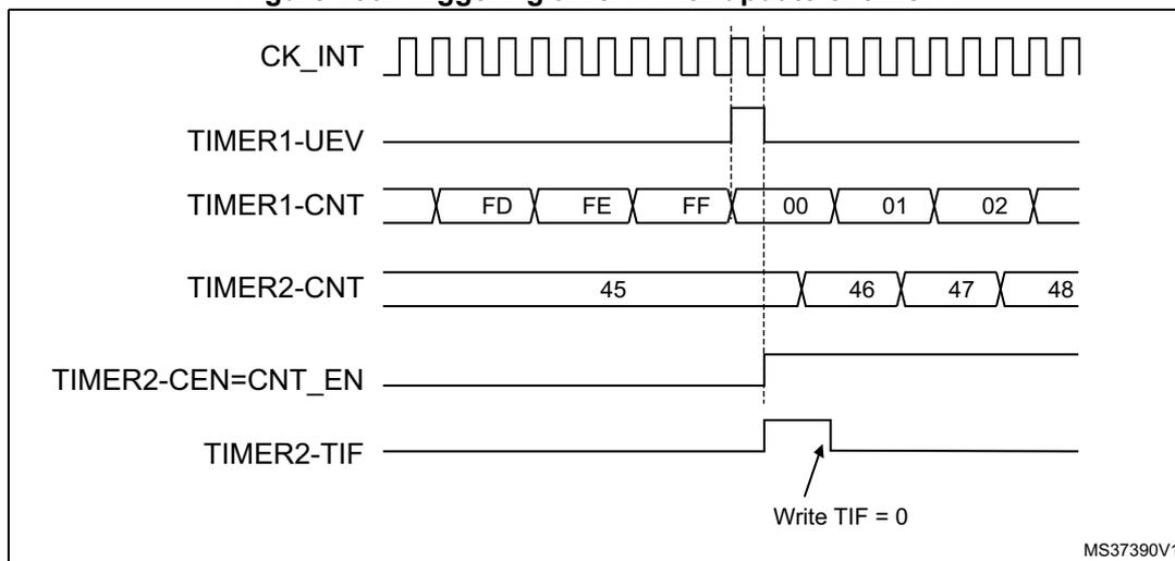
As in the previous example, the user can initialize both counters before starting counting. [Figure 157](#) shows the behavior with the same configuration as in [Figure 156](#) but in trigger mode instead of gated mode (SMS=110 in the TIM2\_SMCR register).
