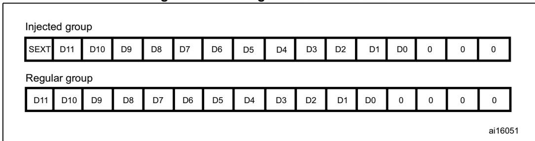
Special case: when left-aligned, the data are aligned on a half-word basis except when the resolution is set to 6-bit. In that case, the data are aligned on a byte basis as shown in [Figure 34](#).
