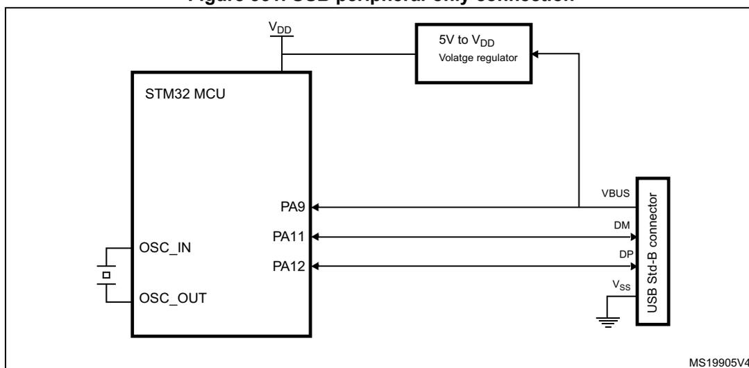
1. Use a regulator to build a bus-powered device.
