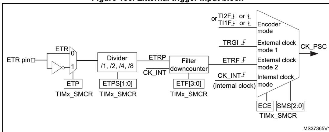
For example, to configure the upcounter to count each 2 rising edges on ETR, use the following procedure:
