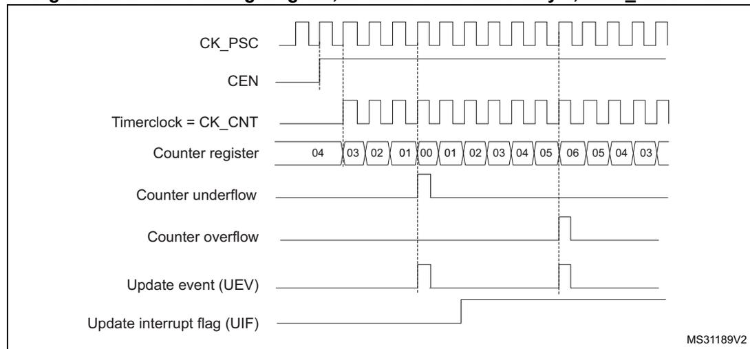
1. Here, center-aligned mode 1 is used (for more details refer to [Section 13.4: TIM1 and TIM8 registers](#)).
