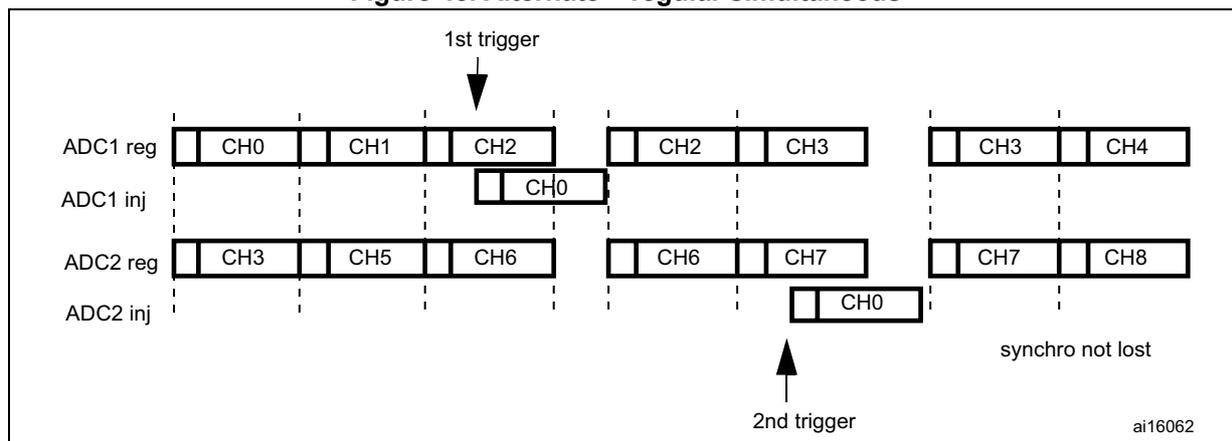
If a trigger occurs during an injected conversion that has interrupted a regular conversion, it is ignored. *Figure 46* shows the behavior in this case (2nd trigger is ignored).
