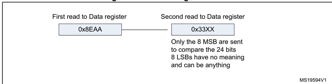
**Figure 269. I<sup>2</sup>S Philips standard (16-bit extended to 32-bit packet frame with CPOL = 0)**
