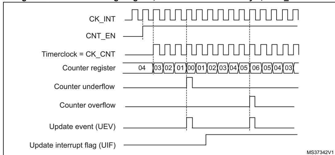
1. Here, center-aligned mode 1 is used, for more details refer to [Section 14.4.1: TIMx control register 1 \(TIMx\\_CR1\)](#).
