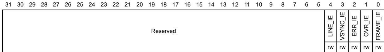
The DCMI\_IER register is used to enable interrupts. When one of the DCMI\_IER bits is set, the corresponding interrupt is enabled. This register is accessible in both read and write.
