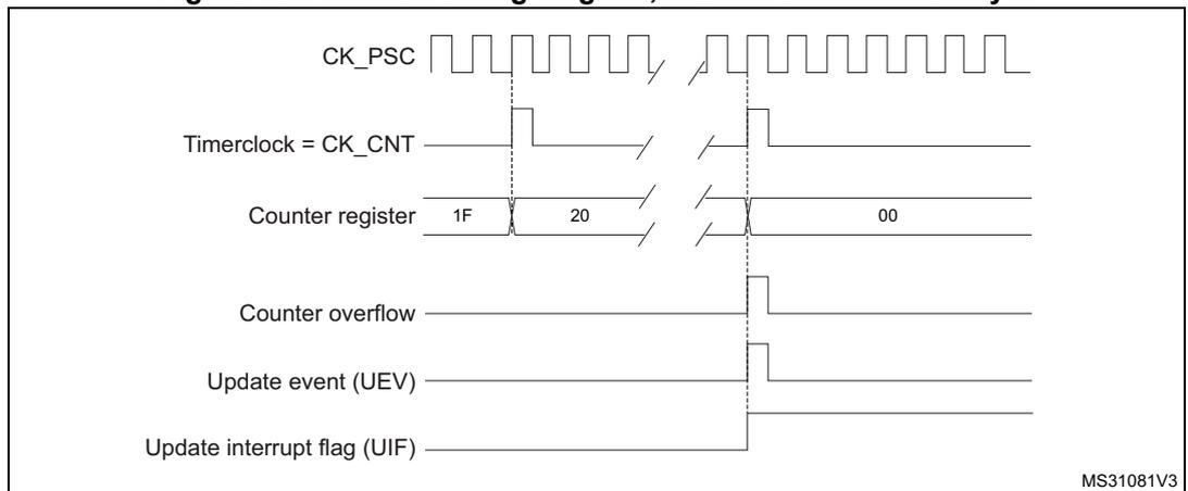
**Figure 167. Counter timing diagram, update event when ARPE=0 (TIMx\_ARR not preloaded)**
