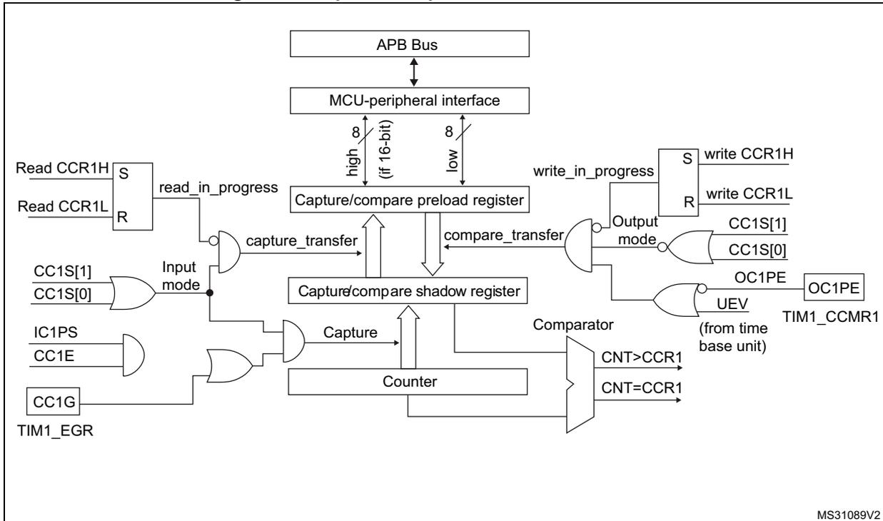
Figure 93. Output stage of capture/compare channel (channel 1 to 3)
