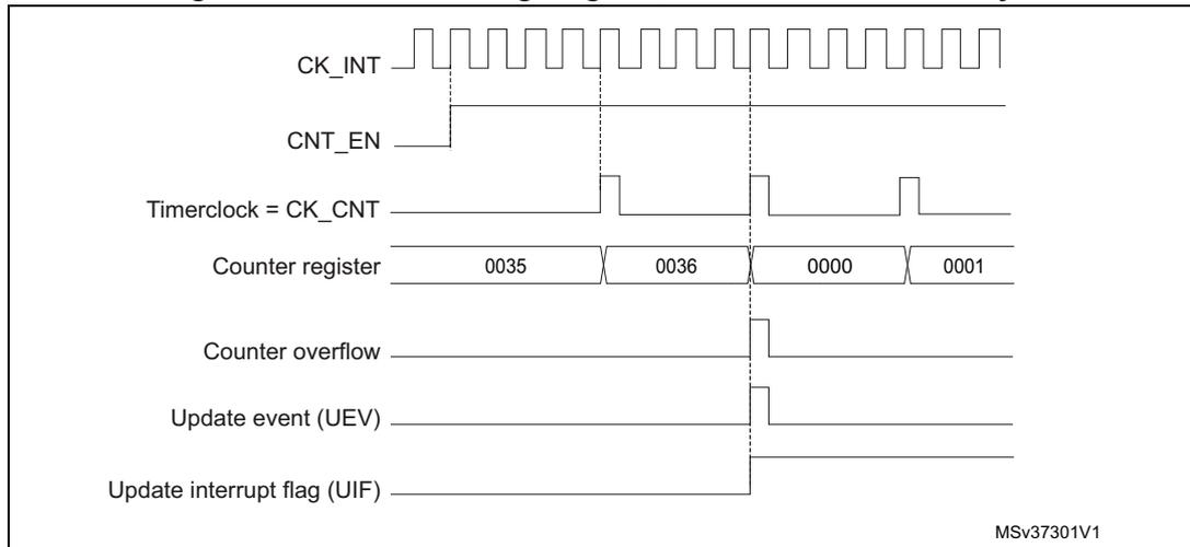
**Figure 119. Counter timing diagram, internal clock divided by N**
