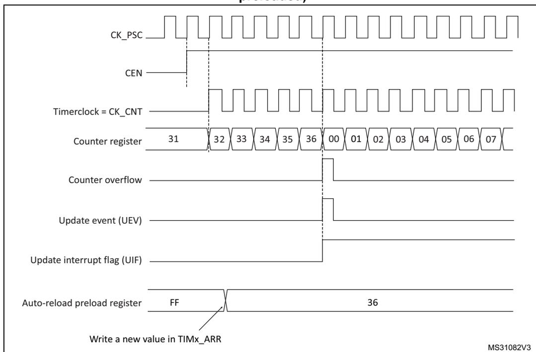
**Figure 168. Counter timing diagram, update event when ARPE=1 (TIMx\_ARR preloaded)**
