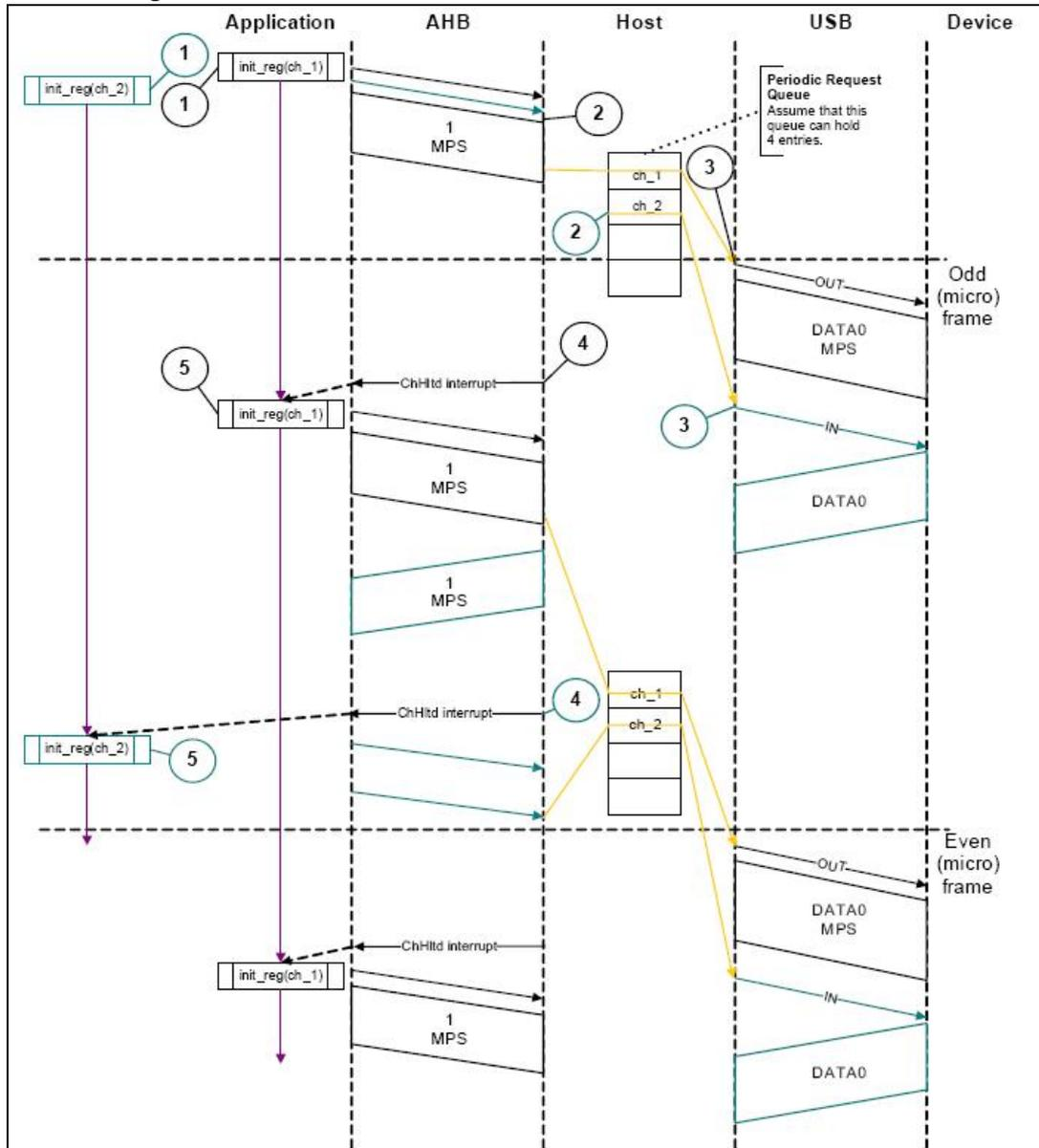
Figure 388. Normal isochronous OUT/IN transactions - Slave mode
