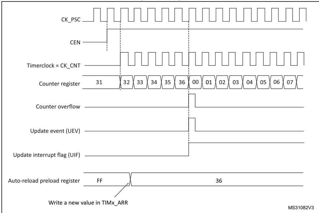
**Figure 73. Counter timing diagram, update event when ARPE=1 (TIMx\_ARR preloaded)**
