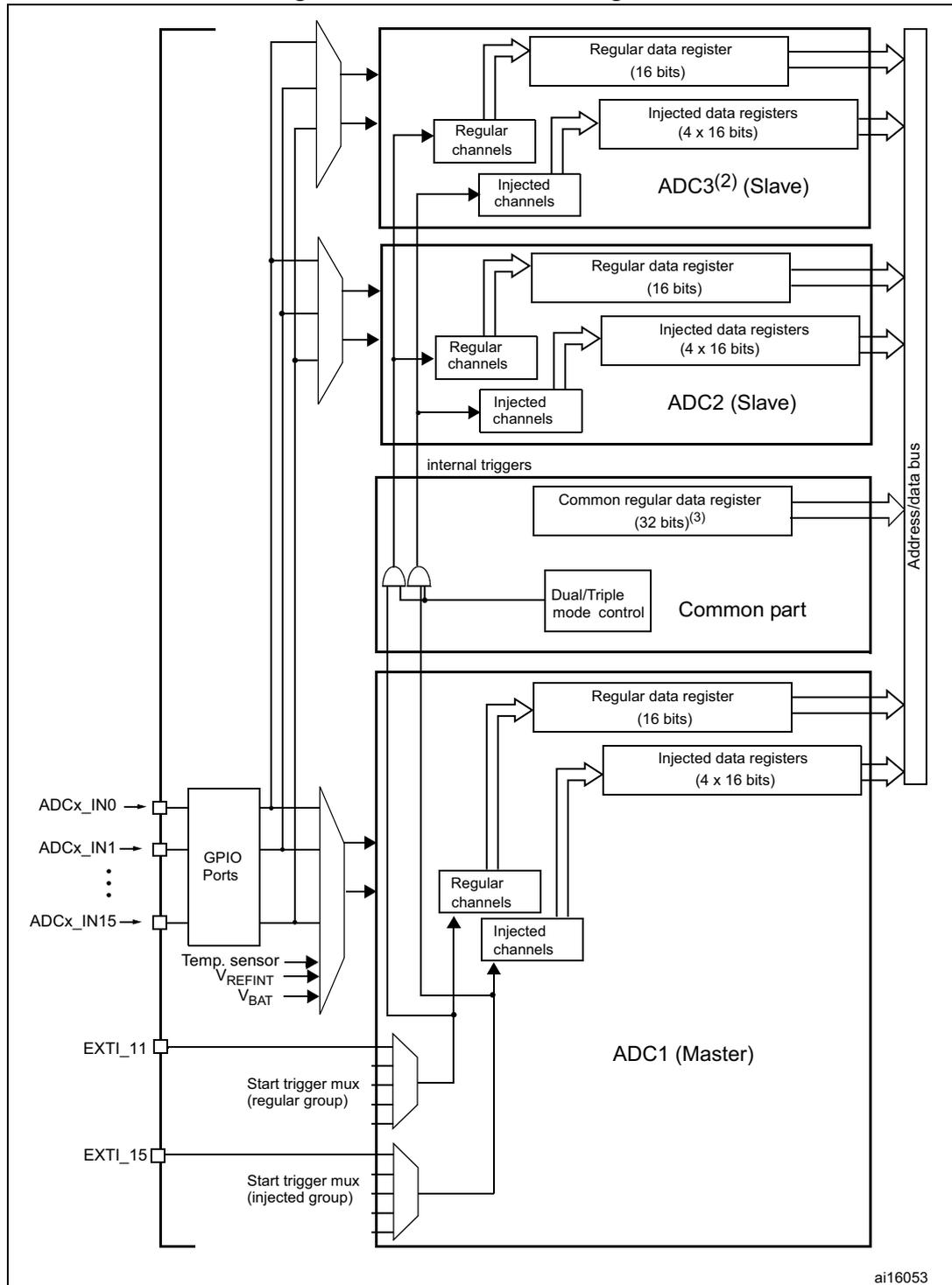
1. Although external triggers are present on ADC2 and ADC3 they are not shown in this diagram.
