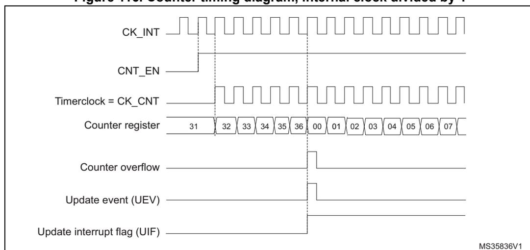
**Figure 117. Counter timing diagram, internal clock divided by 2**
