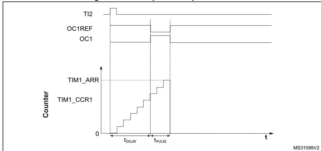
For example the user may want to generate a positive pulse on OC1 with a length of t<sub>PULSE</sub> and after a delay of t<sub>DELAY</sub> as soon as a positive edge is detected on the TI2 input pin.
