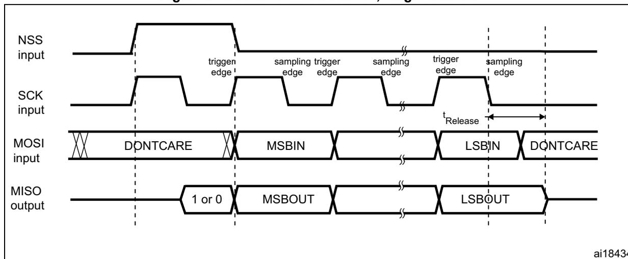
Figure 252. TI mode - Slave mode, continuous transfer
