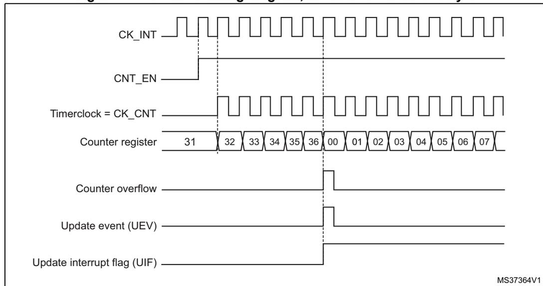
**Figure 186. Counter timing diagram, internal clock divided by 2**
