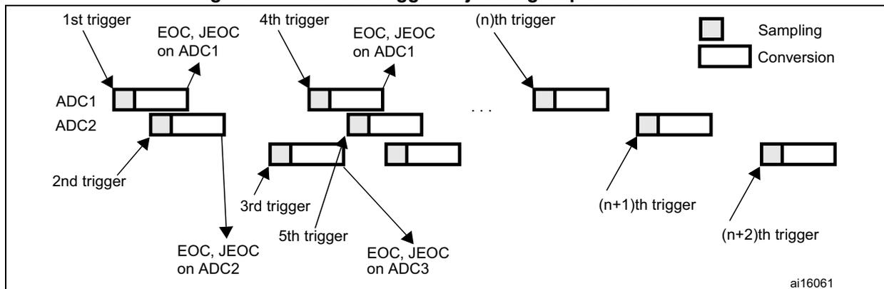
**10.9.5 Combined regular/injected simultaneous mode**
