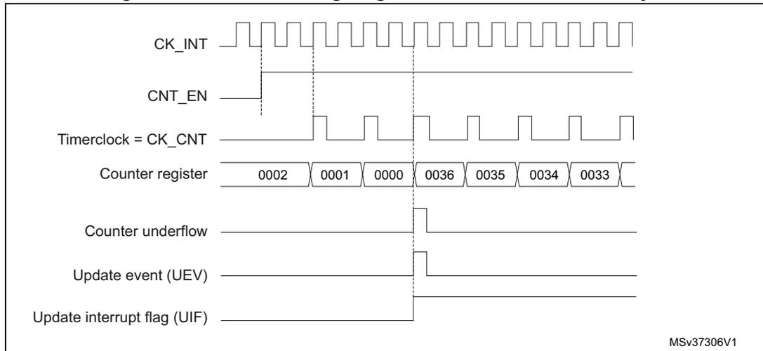
**Figure 124. Counter timing diagram, internal clock divided by 4**
