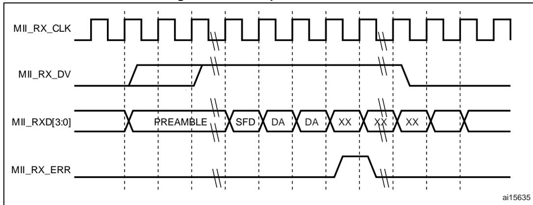
Figure 332. Reception with false carrier indication
