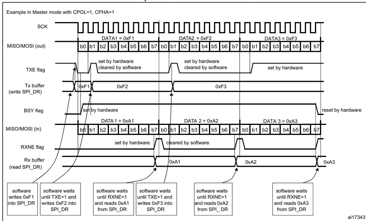
**Figure 256. TXE/RXNE/BSY behavior in Slave / full-duplex mode (BIDIMODE=0, RXONLY=0) in case of continuous transfers**
