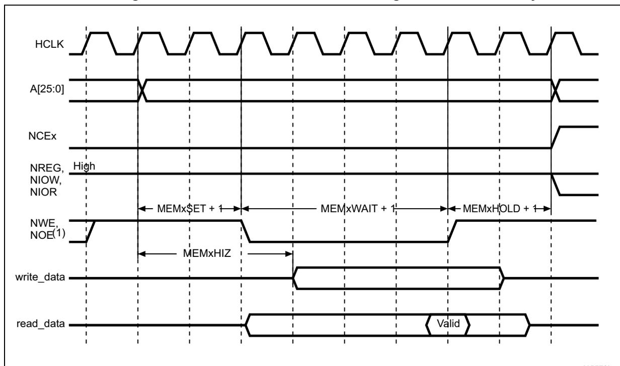
1. NOE remains high (inactive) during write access. NWE remains high (inactive) during read access.
