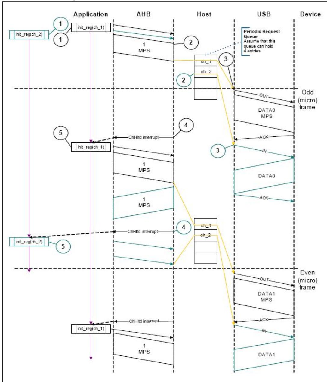
Figure 384. Bulk/control IN transactions - Slave mode
