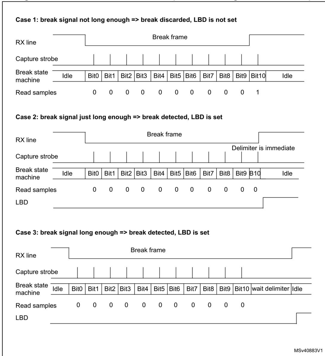
Figure 233. Break detection in LIN mode vs. Framing error detection
