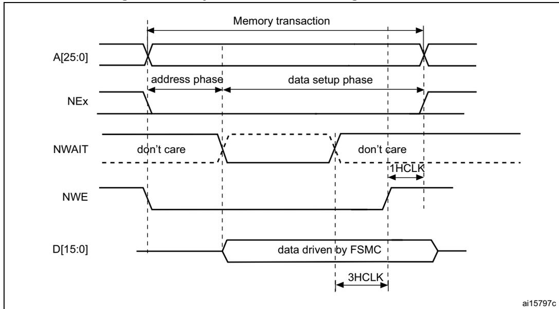
1. NWAIT polarity depends on WAITPOL bit setting in FSMC\_BCRx register.
