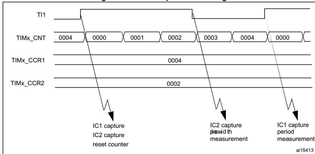
1. The PWM input mode can be used only with the TIMx\_CH1/TIMx\_CH2 signals due to the fact that only TI1FP1 and TI2FP2 are connected to the slave mode controller.
