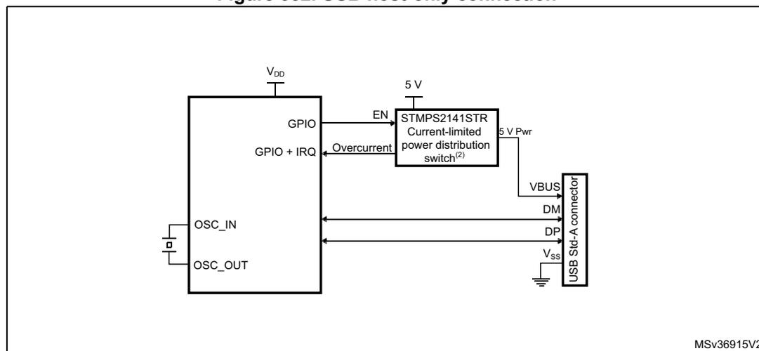
1. STMP52141STR needed only if the application has to support a  $V_{BUS}$  powered device. A basic power switch can be used if 5 V are available on the application board.
