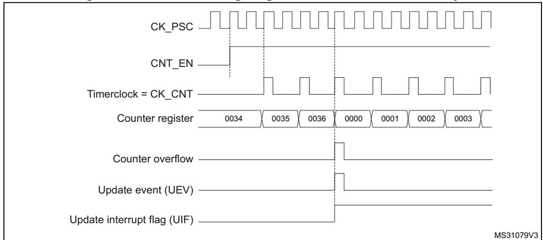
**Figure 165. Counter timing diagram, internal clock divided by 4**
