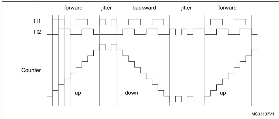
Figure 107 gives an example of counter behavior when TI1FP1 polarity is inverted (same configuration as above except CC1P='1').
