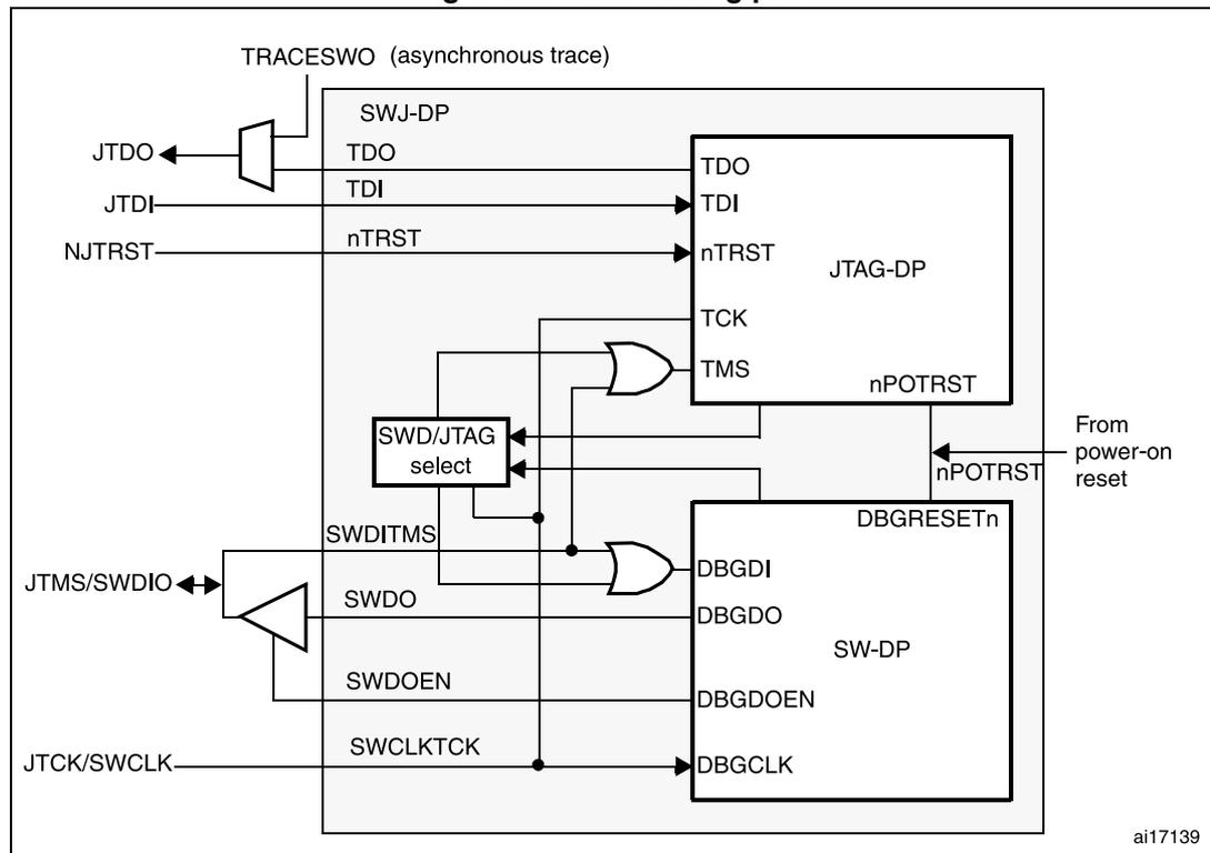
Figure 420 shows that the asynchronous TRACE output (TRACESWO) is multiplexed with TDO. This means that the asynchronous trace can only be used with SW-DP, not JTAG-DP.
