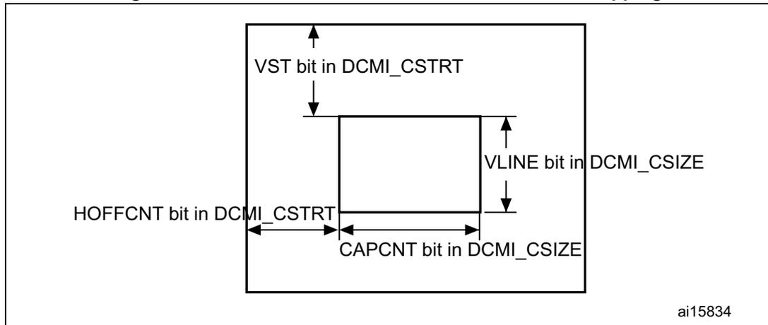
These registers specify the coordinates of the starting point of the capture window as a line number (in the frame, starting from 0) and a number of pixel clocks (on the line, starting from 0), and the size of the window as a line number and a number of pixel clocks. The CAPCNT value can only be a multiple of 4 (two least significant bits are forced to 0) to allow the correct transfer of data through the DMA.
