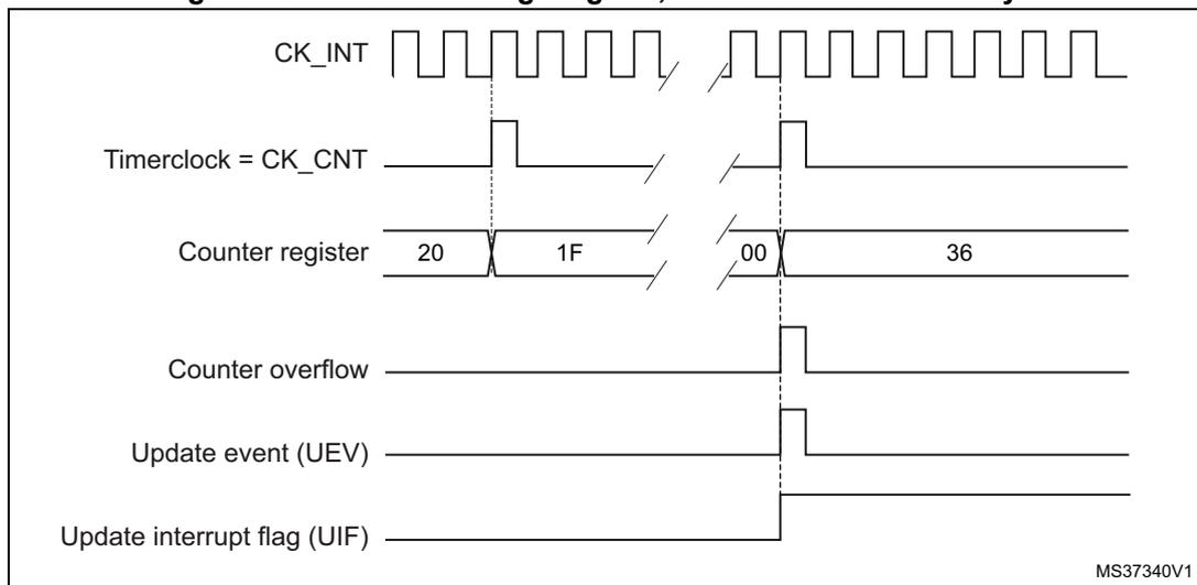
Figure 126. Counter timing diagram, Update event
