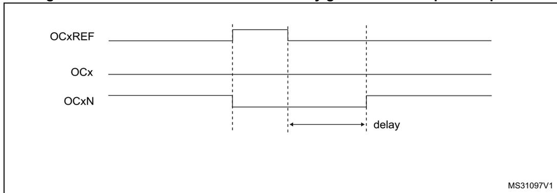
The dead-time delay is the same for each of the channels and is programmable with the DTG bits in the TIMx\_BDTR register. Refer to [Section 13.4.18: TIM1 and TIM8 break and dead-time register \(TIMx\\_BDTR\)](#) for delay calculation.
