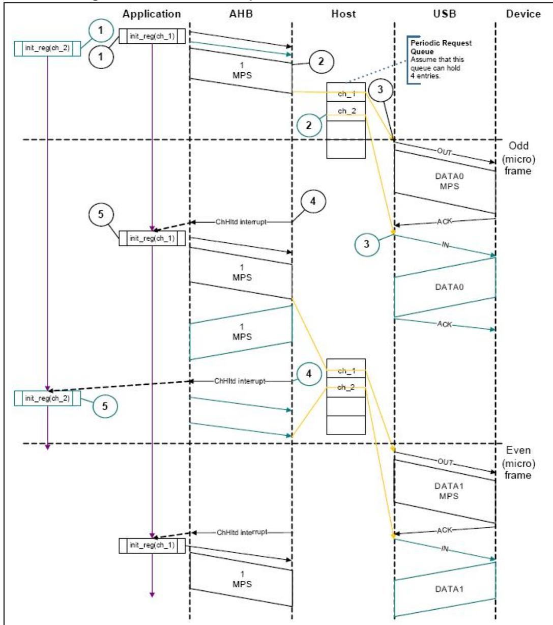
Figure 386. Normal interrupt OUT/IN transactions - Slave mode
