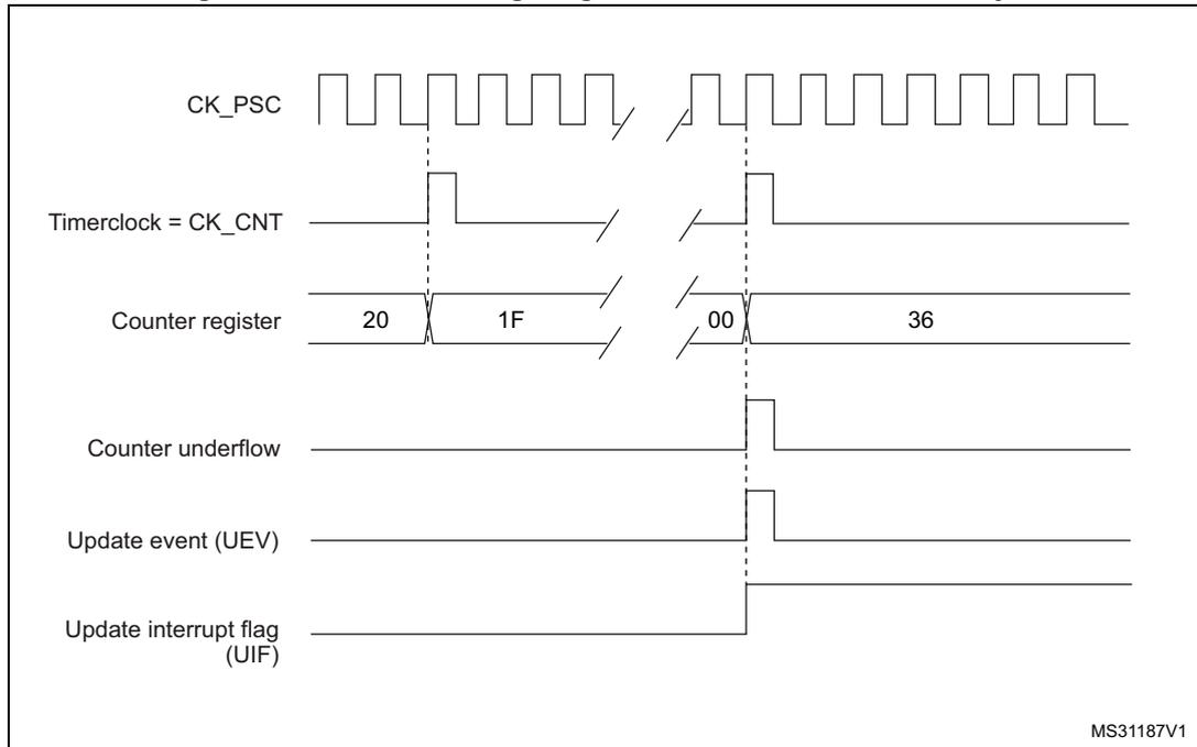
Figure 78. Counter timing diagram, update event when repetition counter is not used
