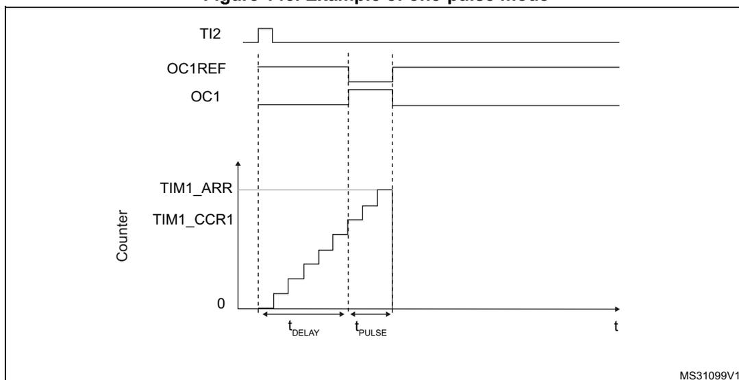
For example the user may want to generate a positive pulse on OC1 with a length of  $t_{PULSE}$  and after a delay of  $t_{DELAY}$  as soon as a positive edge is detected on the TI2 input pin.
