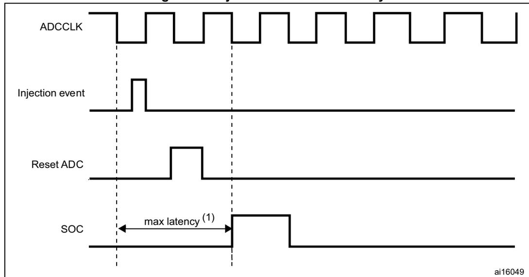
1. The maximum latency value can be found in the electrical characteristics of the STM32F20x and STM32F21x datasheets.
