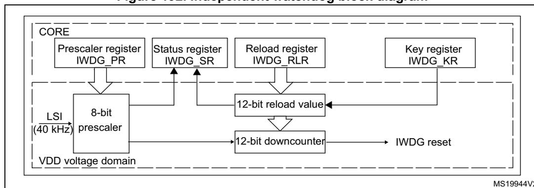
Note: The watchdog function is implemented in the  $V_{DD}$  voltage domain, still functional in Stop and Standby modes.
