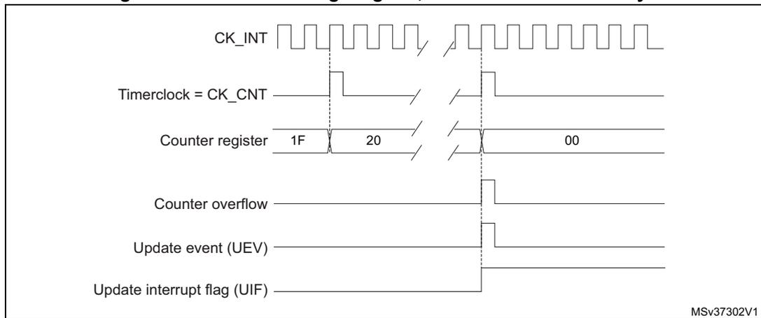
**Figure 120. Counter timing diagram, Update event when ARPE=0 (TIMx\_ARR not preloaded)**
