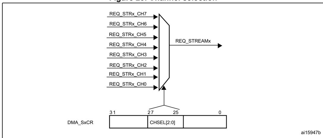
The 8 requests from the peripherals (TIM, ADC, SPI, I2C, etc.) are independently connected to each channel and their connection depends on the product implementation.
