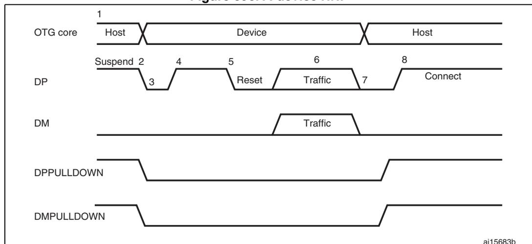
1. DPPULLDOWN = signal from core to PHY to enable/disable the pull-down on the DP line inside the PHY.
