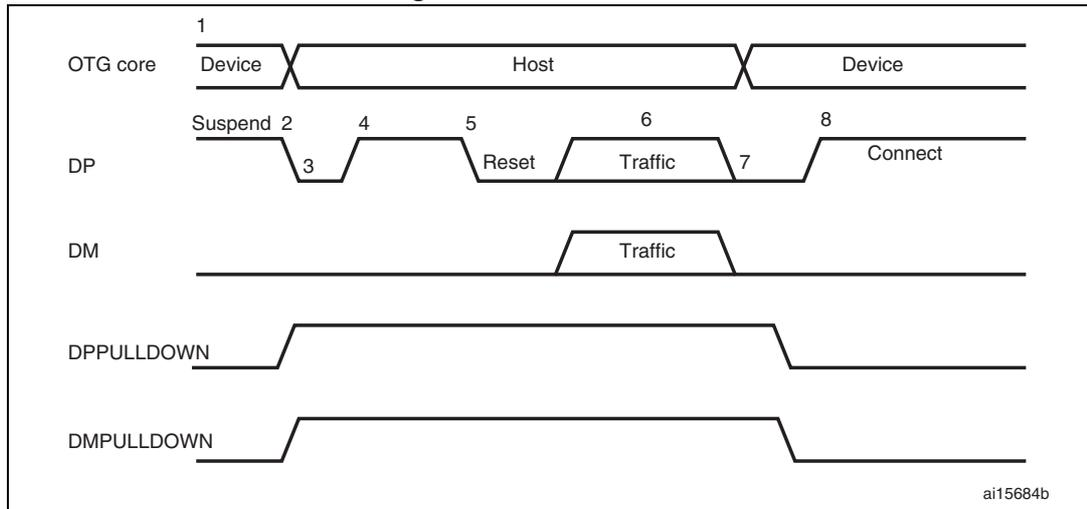
1. DPPULLDOWN = signal from core to PHY to enable/disable the pull-down on the DP line inside the PHY. DMPULLDOWN = signal from core to PHY to enable/disable the pull-down on the DM line inside the PHY.
