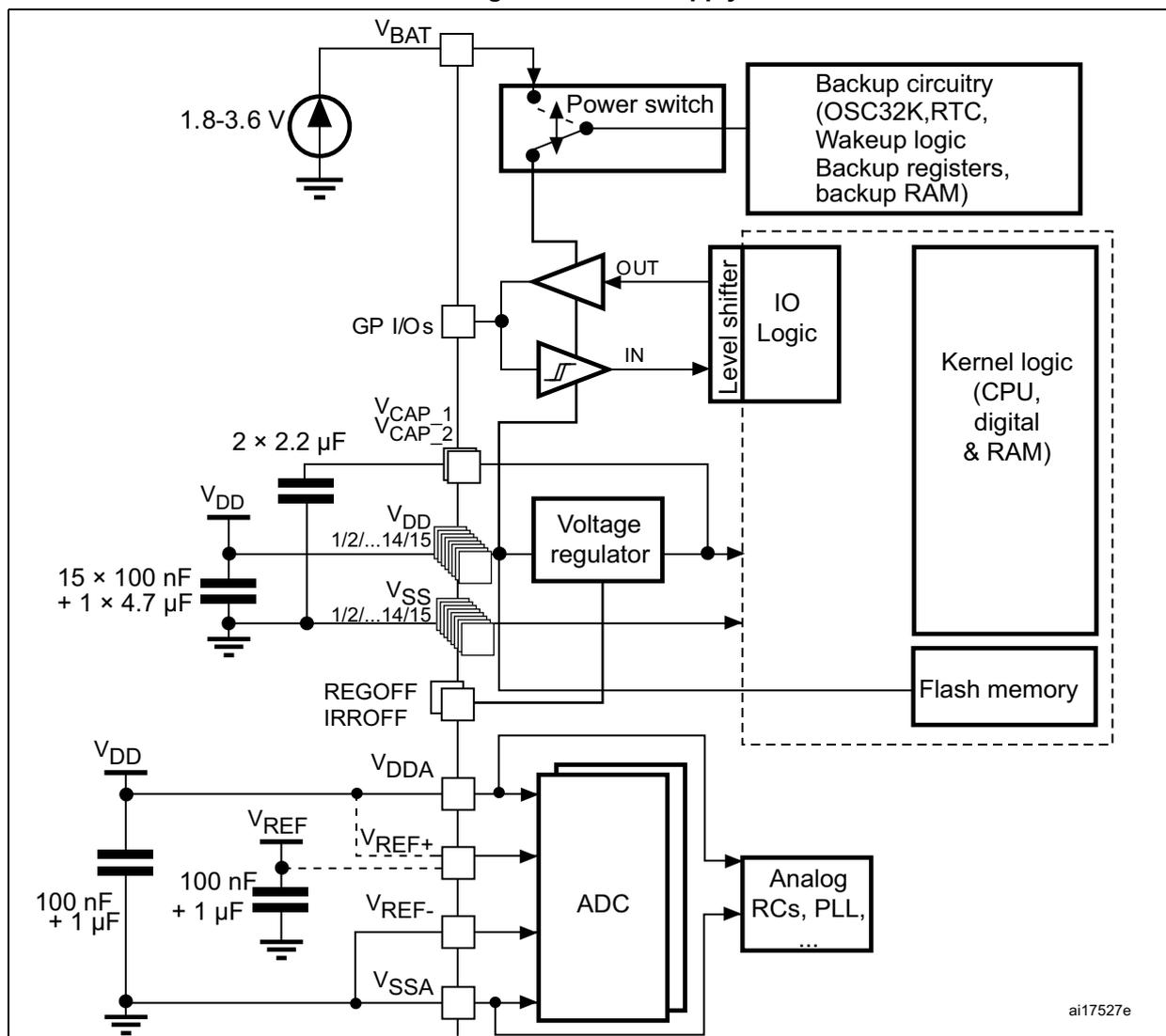
1.  $V_{DDA}$  and  $V_{SSA}$  must be connected to  $V_{DD}$  and  $V_{SS}$ , respectively.
